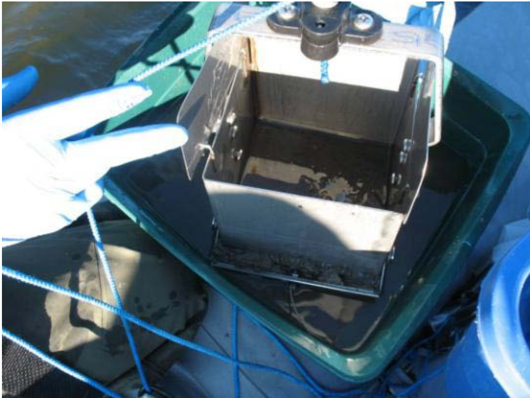
Photograph 4-3 Good Sediment Sample (Ekman Grab Sample with Jaws fully Closed)
