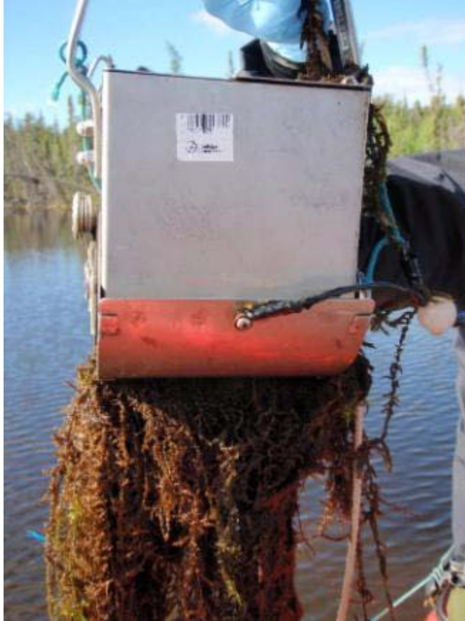
Photograph 4-2 Poor Sediment Sample (Ekman Grab Sample with Jaws not fully Closed)
